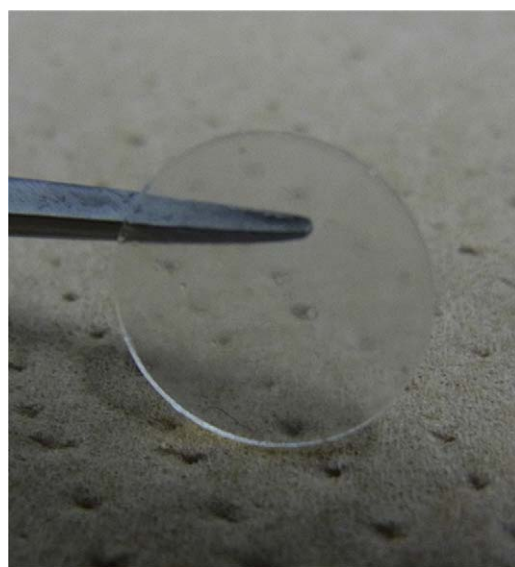
Fig. 2. Photograph of vacuum degassed solid-state electrolyte pellet.
